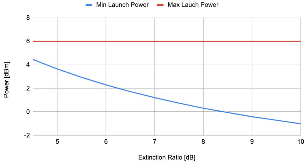
Figure 4 - Acceptable ONU Launch Power at 2.5Gb/s
