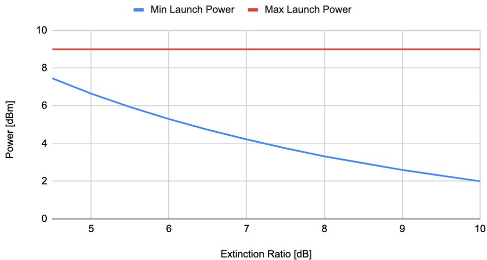
Figure 3 - Acceptable ONU Launch Power at 10Gb/s
