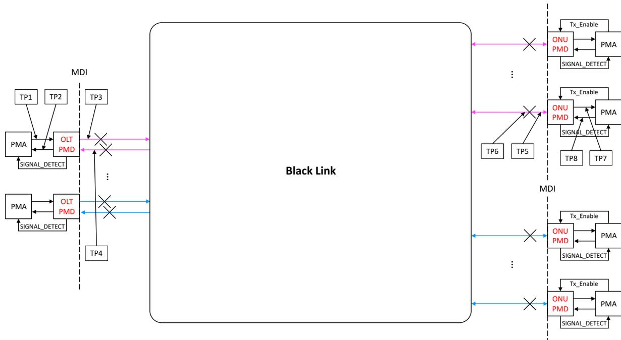
Figure 2 - Super-PON PMD Test Points
