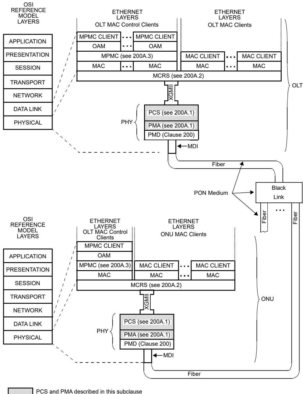
**Figure 200A-1—Relationship of EPON P2MP PMD to the ISO/IEC OSI reference model and the IEEE 802.3 Ethernet model**
