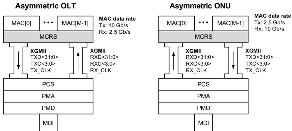
**Figure 200A-3—Asymmetric OLT and ONU layering diagram**
