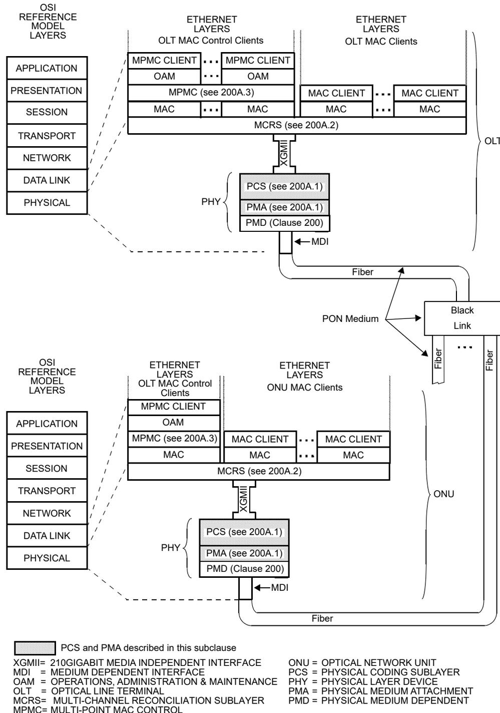
**Figure 200A-1—Relationship of EPON P2MP PMD to the ISO/IEC OSI reference model and the IEEE 802.3 Ethernet model**
