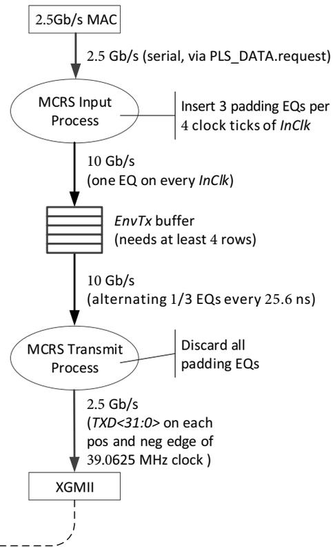
Figure 200A-4—Upstream channel operating at 2.5 Gb/s
