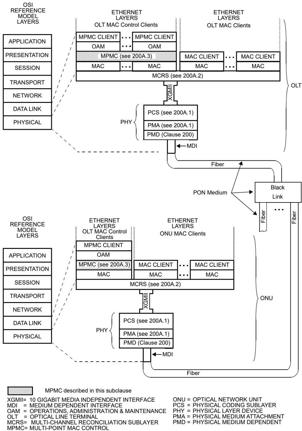
**Figure 200A-5—Relationship of EPON P2MP PMD to the ISO/IEC OSI reference model and the IEEE 802.3 Ethernet model**
