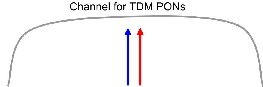
Burst on wavelength drift much less than the filter bandwidth
