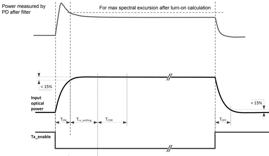
Figure 200C-2 - A potential power envelope output after filtering
