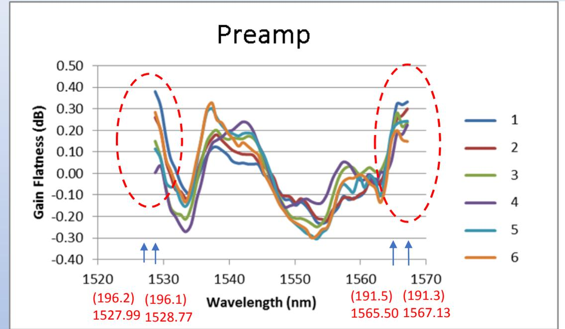
Figure 5, Gain Flattened Preamp
