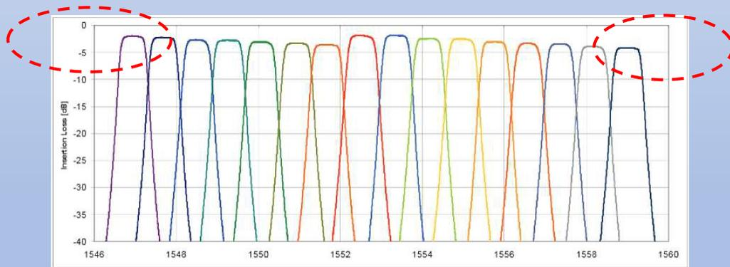
Figure 1, Typical Flat-top Filter
