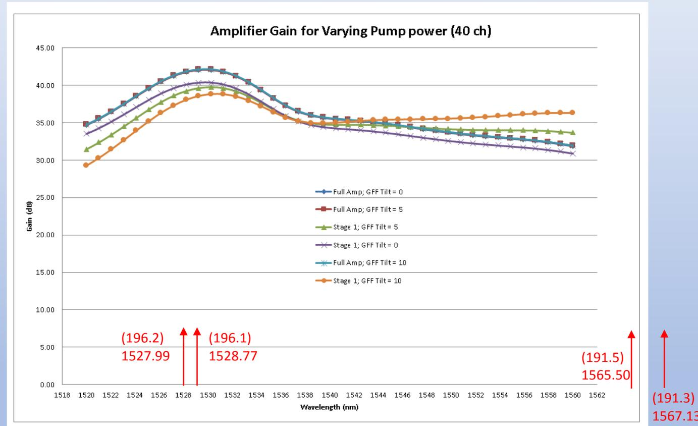
Figure 3, Erbium Fiber Gain and Tilt
