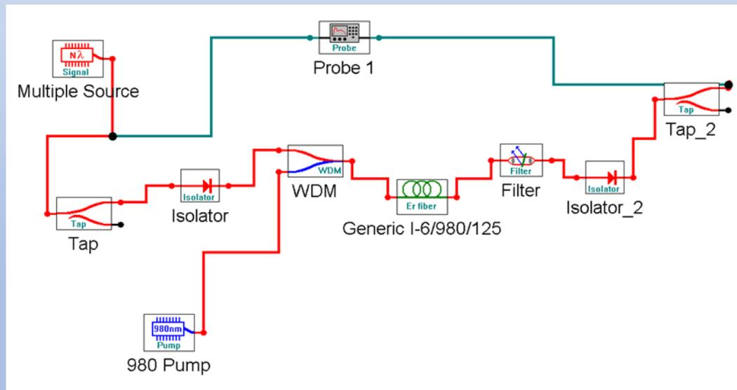
Figure 2, Optical Amplifier Block Diagram
