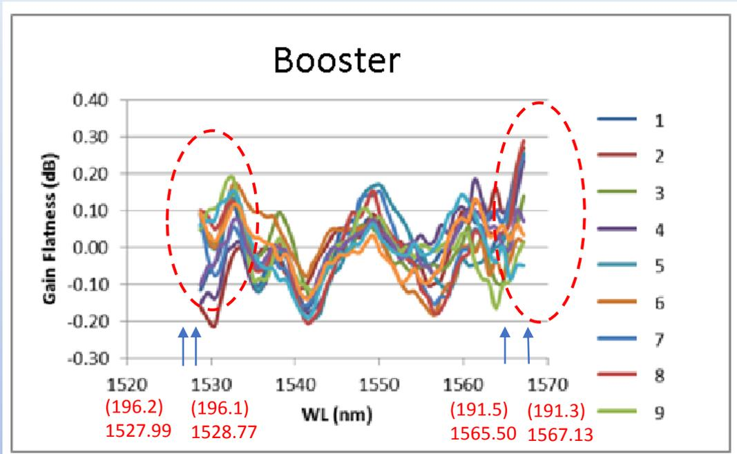
Figure 4, Gain Flattened Booster
