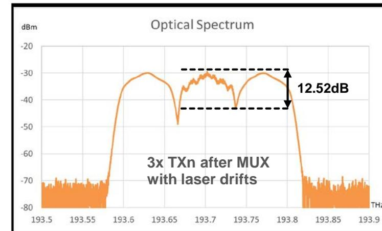
The dip level clearly shows that (a)  $TW_n$  signals have less inter-channel Xtalk than  $TW_w$ ; and (b) Xtalk increases after 3 laser frequency shifts
