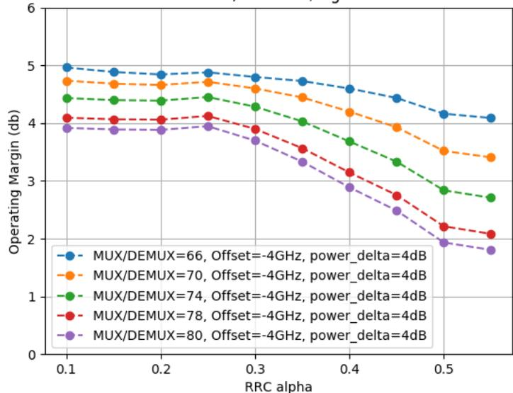
Tx crosstalk test: RRC center, RRC0.4 Left/Right: RxOSR1.15 RxBW34GHz
