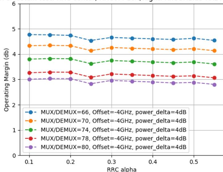
RX test: RRC center and Left/Right channels: RxOSR1.15 RxBW34GHz
