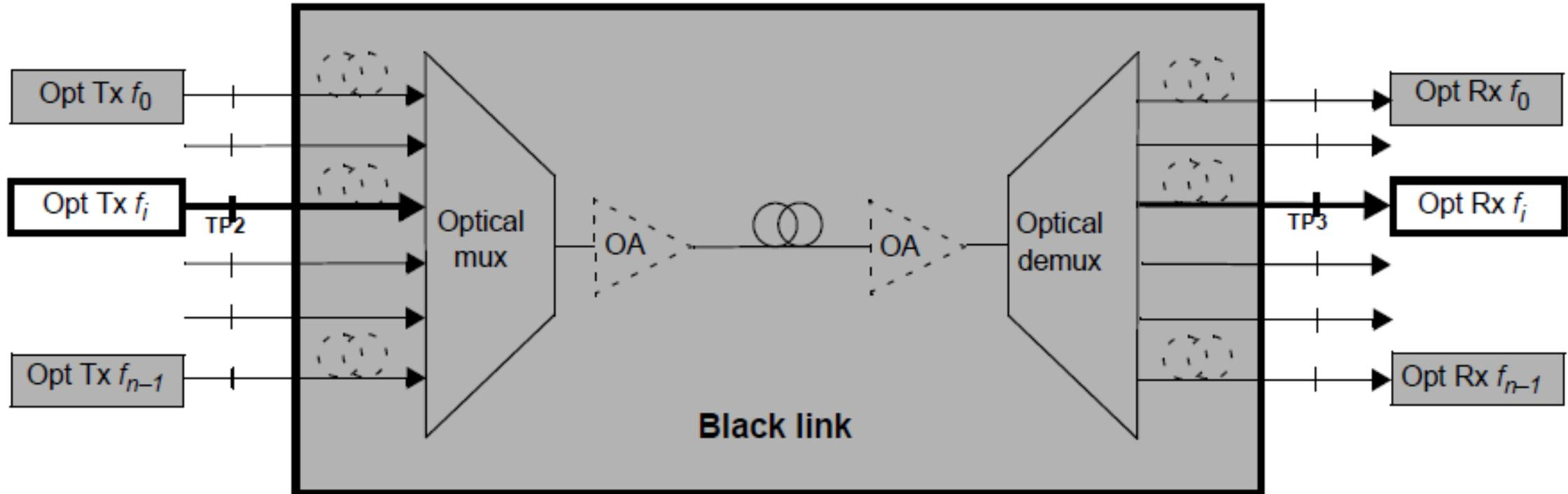
Fully consistent with Figure 5-1 in G.698.2. The transmitter frequency is used instead of transmitter wavelength, no OADM is shown, and “black link” is referred to instead of “DWDM link”.
