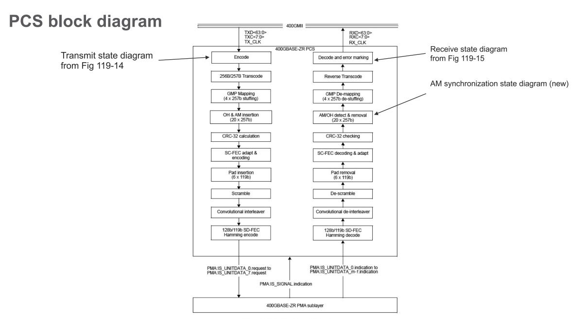
Figure 155-2-Functional block diagram
