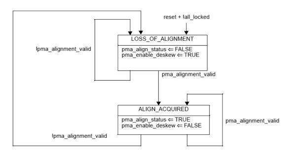
Figure 155-14—PMA deskew state diagram
