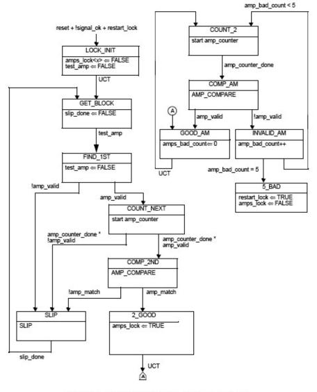
Figure 155-15-Alignment marker lock state diagram
