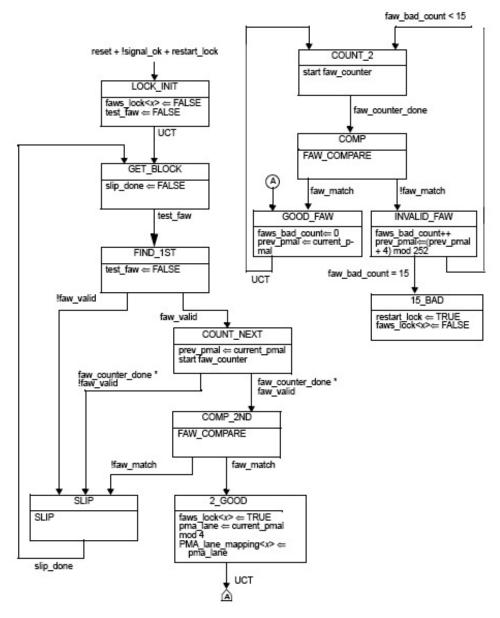
Figure 155-13-DSP FAW synchronization state diagram
