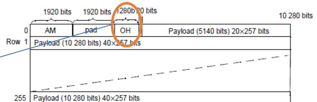
Figure 155-4 400GBASE-ZR frame structure
