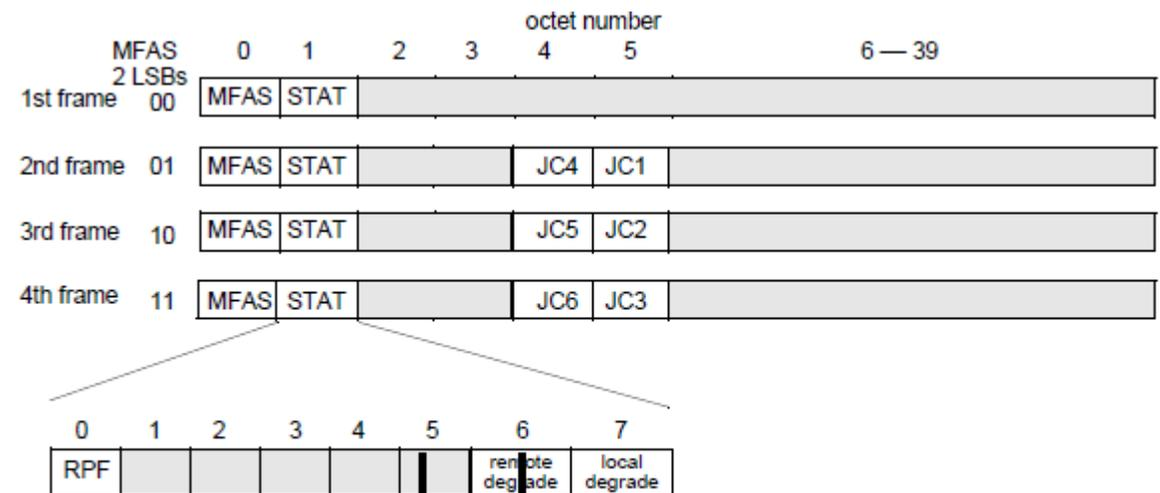
Figure 155-5—Contents of OH fields in four-frame multi-frame
