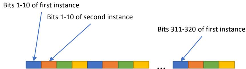
Construction of OH field within the 400GBASE-ZR frame
