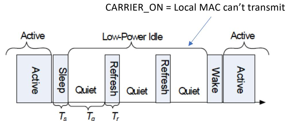
**Figure 78–3—Overview of EEE LPI operation**
