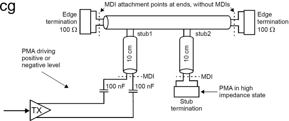
Figure 147-20—Multidrop line termination and PMA
