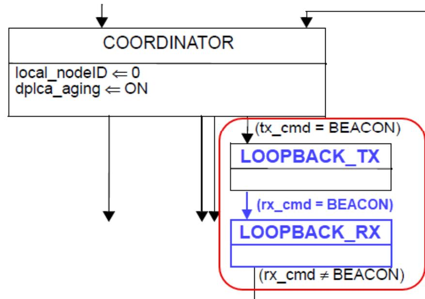
(Only the relevant portion of the D-PLCA Control State Diagram (Figure 148-8) shown)
