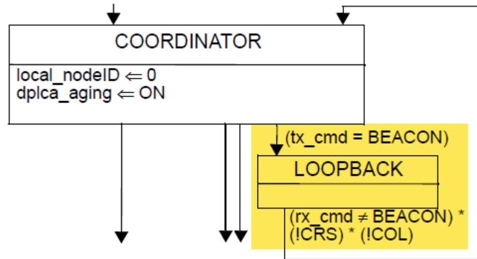
(Only the relevant portion of the D-PLCA Control State Diagram (Figure 148-8) shown)
