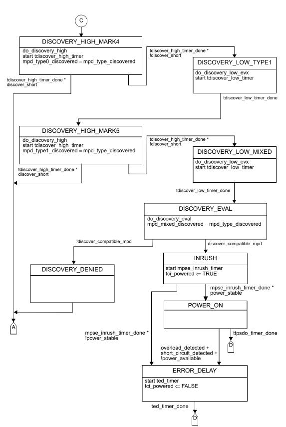
Figure 169-4-Top level MPSE state diagram, part b
