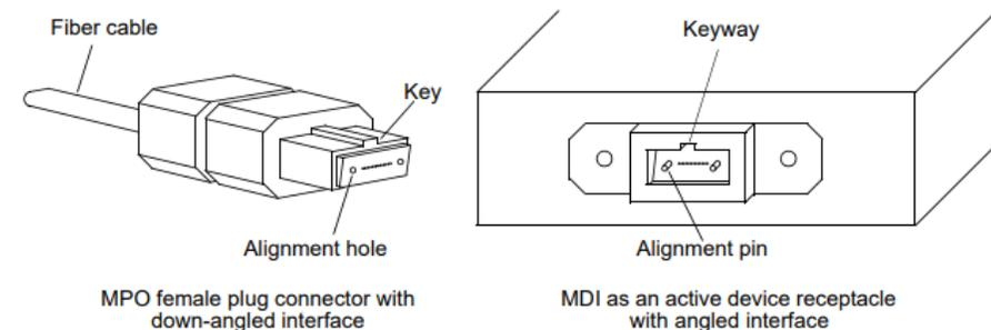
Figure 167-9—MPO female plug with down-angled interface and MDI active device receptacle with angled interface
