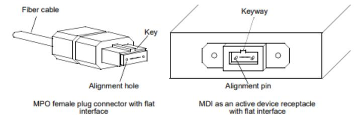
Figure 167-11—MPO female plug with flat interface and MDI active device receptacle with flat interface
