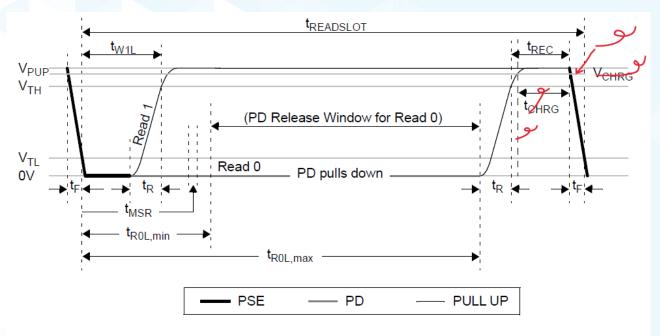
Figure 104-12—Read 0/1 slot timing diagram
