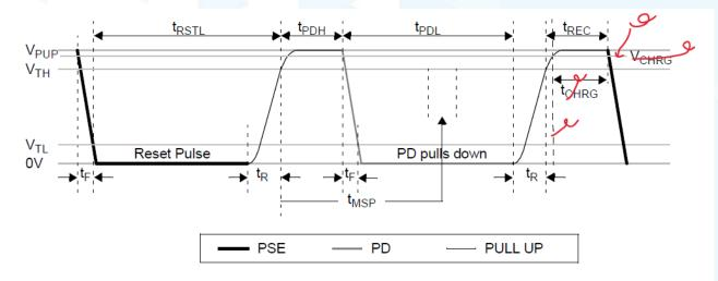
Figure 104–10—Reset command timing diagram
