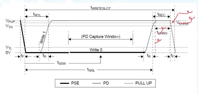
Figure 104–11—Write 0/1 slot timing diagram
