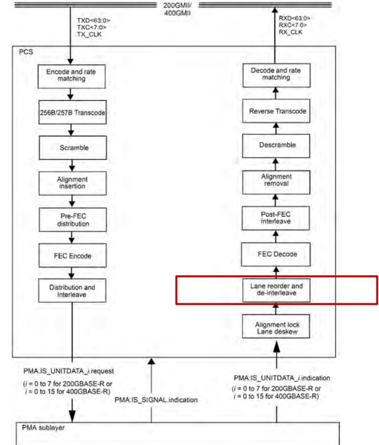
Figure 119-2—Functional block diagram
