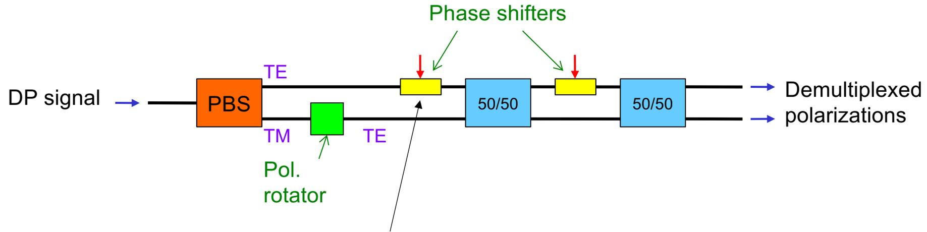
This phase shift requirement is unlimited so will need to reset it, interrupting traffic
