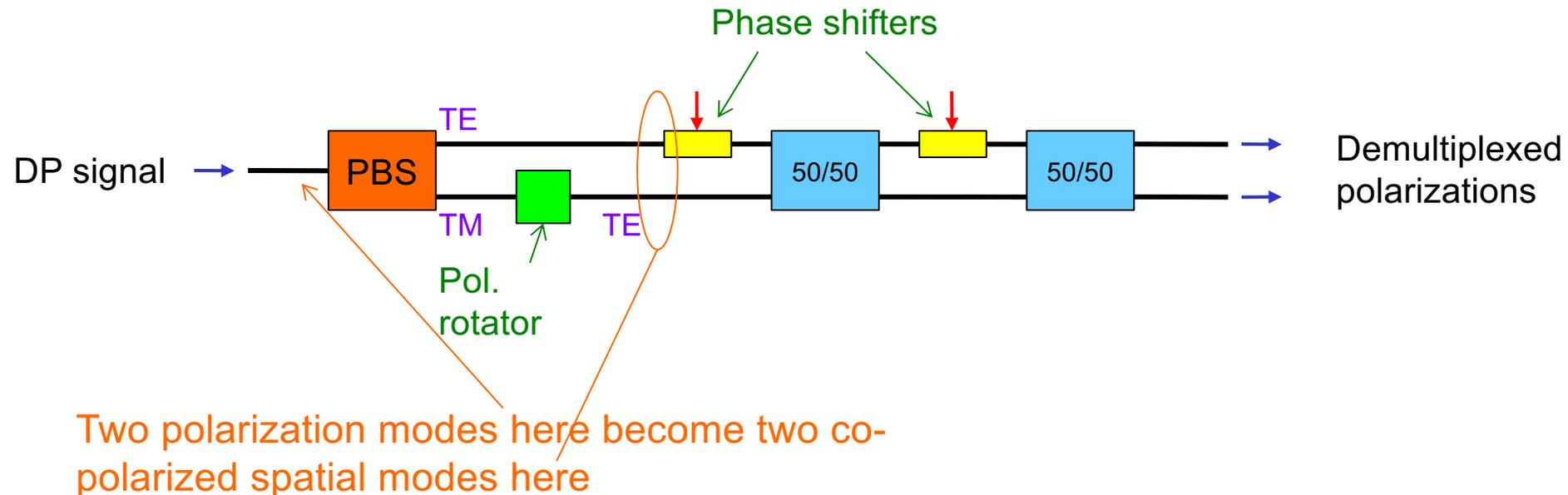
Two phase shifter controls are enough to transfer any input polarization to horizontal or vertical polarization (the other signal will stay orthogonal)
