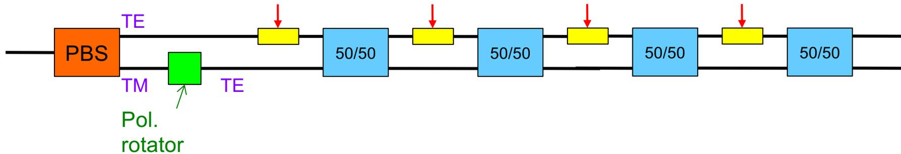
While one phase shifter is resetting gradually back to its center, the other three can keep controlling the polarization
