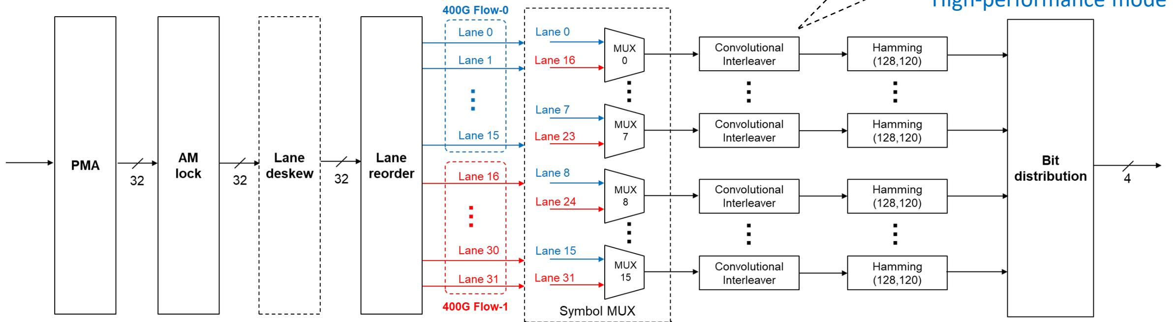
One ASIC to support High-performance or ultra-low latency mode by configurable interleaver.
