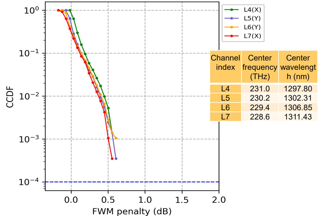
□ Even under the worst-case alignment of ZDW and laser frequencies, the FWM-induced “outage” is  $<10^{-3}$  for a 1dB penalty and a signal launch power of 5dBm per channel.
