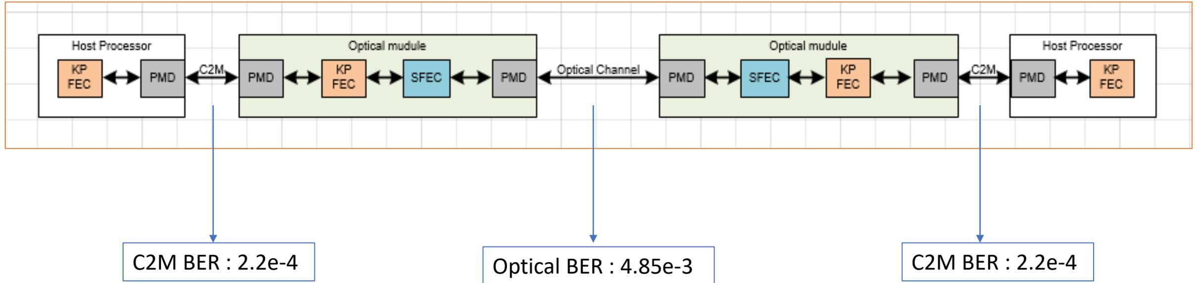
For some of the stringent high loss AUI Channels on the host, we may need to turn on the segmentation FEC proposal to close the link budget.
