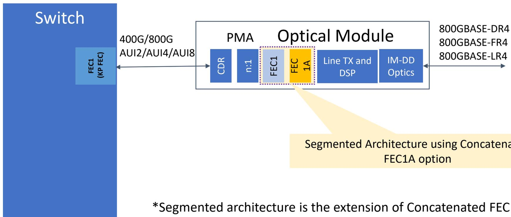
\*Segmented architecture is the extension of Concatenated FEC architecture.
