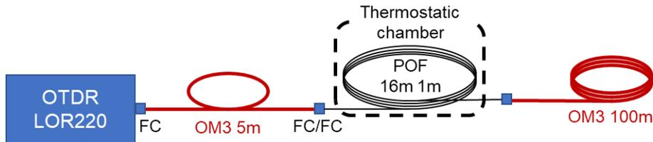
Since the most likely causes of noise are backscattered light and forward scattered light, I re-checked optical time-domain reflection.
