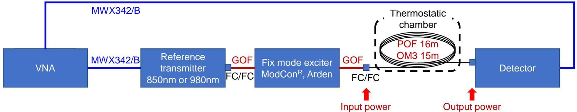
I evaluated the reproducibility of the frequency response measurement with OM3(15m) for reference. Furthermore, I measured the input and output light intensity of OM3 and POF.
