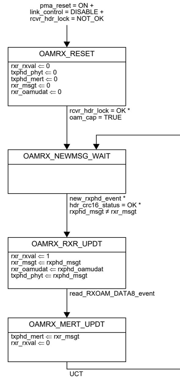
Figure 115–43—PHY 1000BASE-H OAM receive control state diagram
