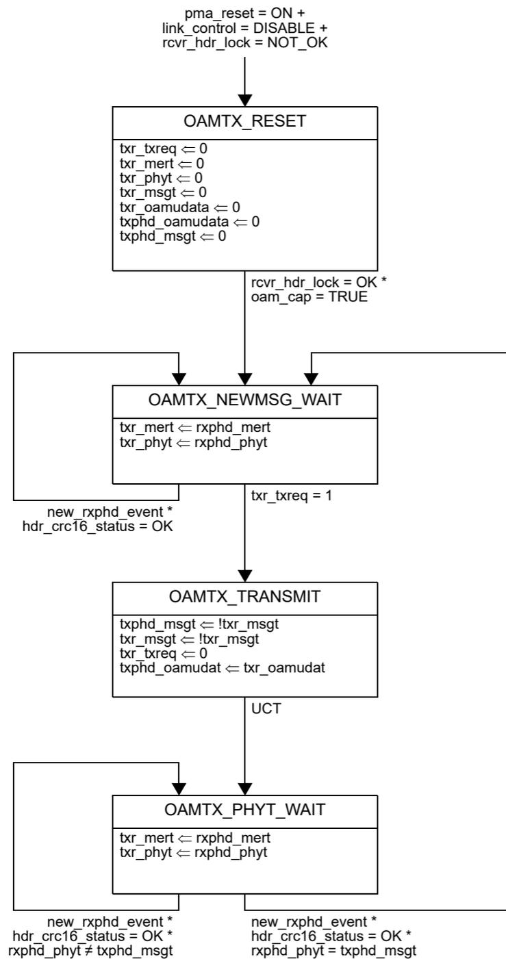
Figure 115–42—PHY 1000BASE-H OAM transmit control state diagram
