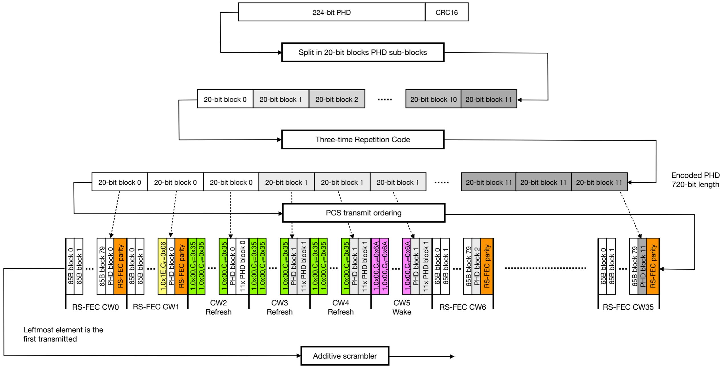
Transmit block, composed by 36 RS codewords, 195840 bits
