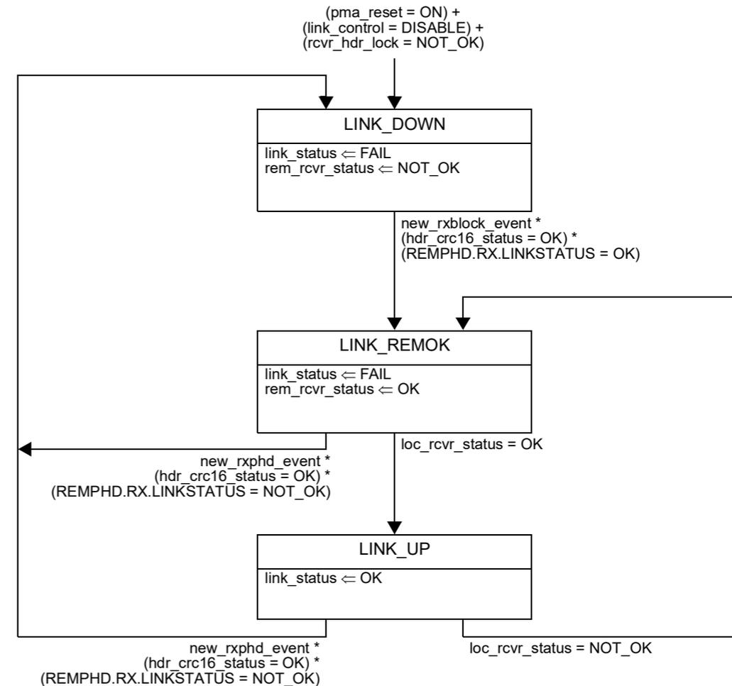
Figure 166–25—Link monitor state diagram
