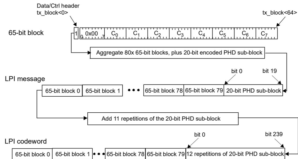
Figure 166–30—LPI codeword transmission
