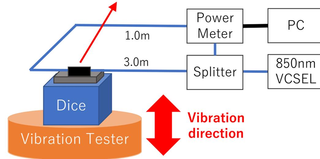
Fig 2, Schematic diagram of vibration test
