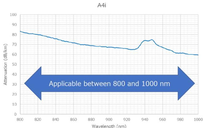
Because perfluorinated polymer has no C-H bond, GI-POF (A4i fiber) has low attenuation between 800 and 1000 nm comparing to conventional SI-POF. 802.3cz PHY (980nm) and 850nm PHY is applicable with GI-POF.
