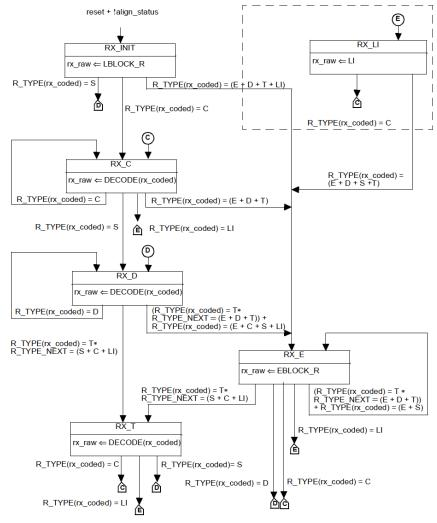
NOTE—Optional state (inside the dotted box) and transition E are only required to support EEE capability.
