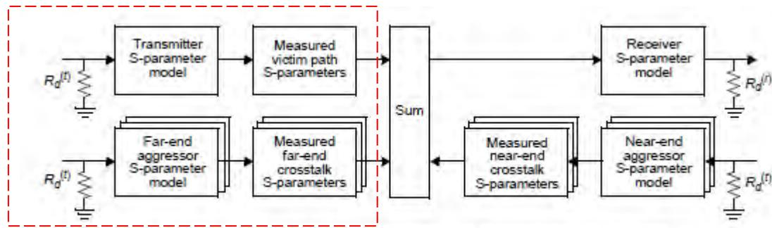
Figure 178A-1—Channel considered for the calculation of COM
