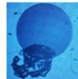
Contaminated fiber connectors commonly seen at both optical module and ODF:
