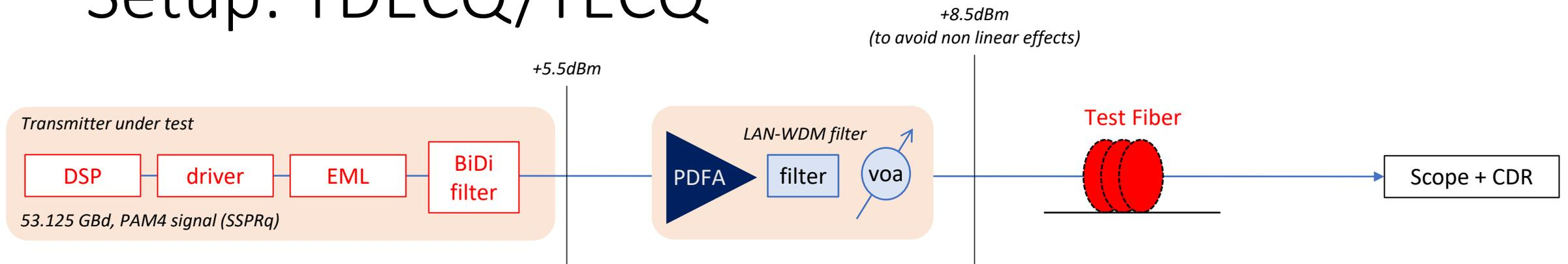
DSP: digital signal processing, EML: external modulated laser, VOA: variable optical attenuator, CDR: Clock and Data recovery, TDECQ: Transmitter and Dispersion Eye Closure Quaternary, TECQ: Transmitter Eye Closure Quaternary
