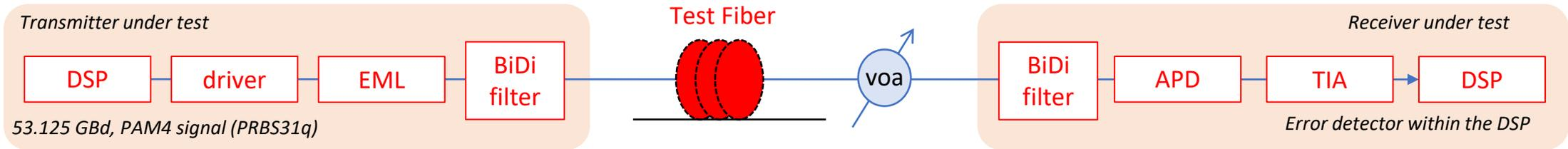
DSP: digital signal processing, EML: external modulated laser, VOA: variable optical attenuator, APD: Avalanche PhotoDiode, TIA: trans-impedance amplifier
