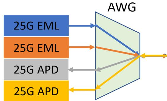
Insertion loss:  $\sim > 3\text{dB}$
