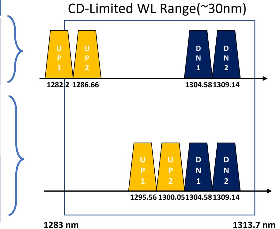
This wavelength plan example takes into account the LWMD wavelength and allows for flexible adjustments within the CD-limited WL range.
