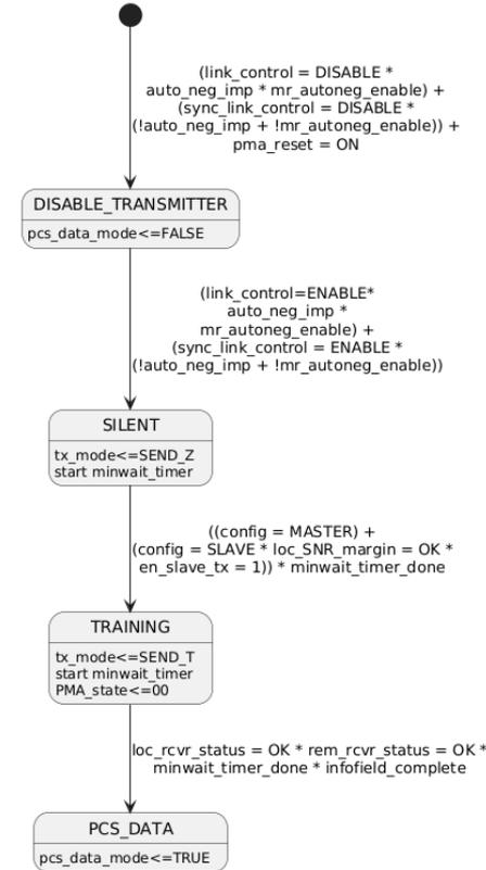
Figure: 100M PHY Control state diagram
