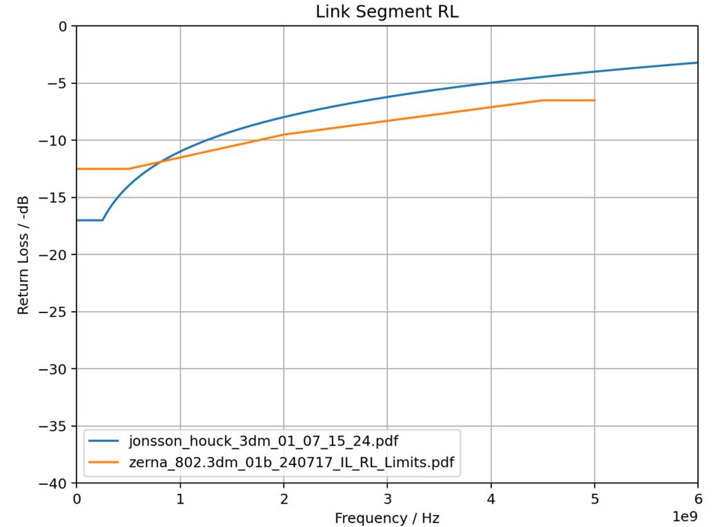
Calculation based on 3m CX174d and 12m CX44a would improve the IL! However, coefficients need adaptation in the low frequencies.
