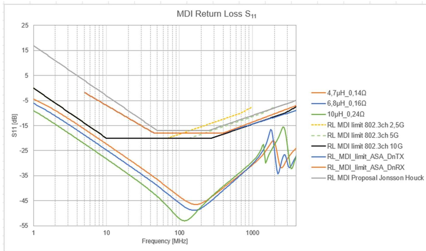
Measured with Vector Network Analyzer (VNA)
