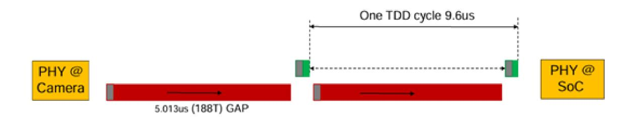
The burst resync headers are shown in the grey blocks at the beginning of the bursts
