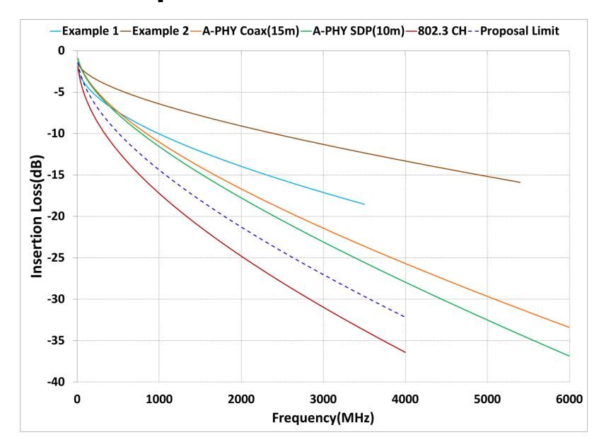
Also propose that upper frequency of limit stop at the data rate chosen. For example, if 2.5 Gb/s camera used then limit stops at 1 GHz like the 802.3ch.
