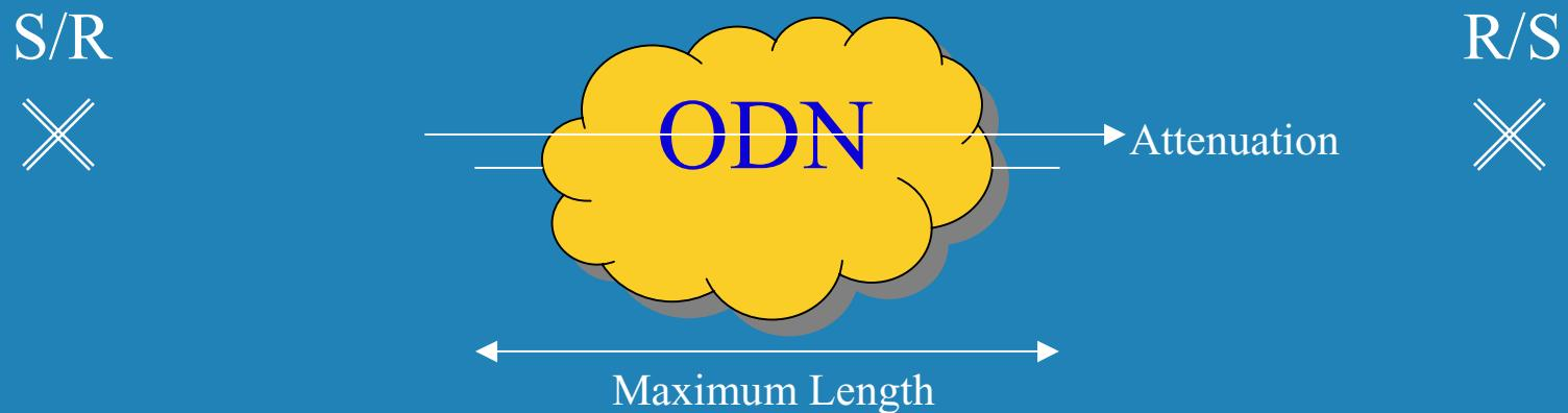
Optical Path Penalty. Df: The difference in apparent link budget between a link that contains only loss (back to back measurement) and a link that contains the maximum optical impairment (e.g. maximum length, worst wavelength, etc.)
