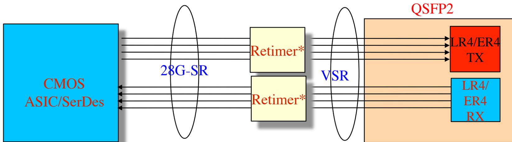
\*Assuming in the case of QSFP2 the retimers are external it solves the power issue and distance
