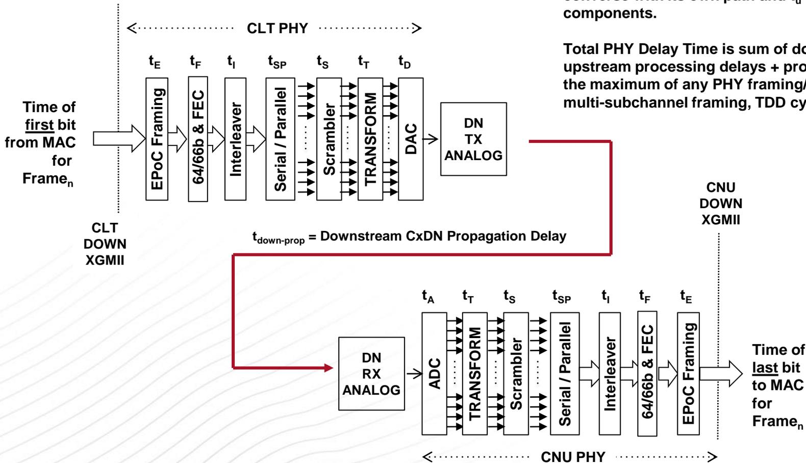
Downstream is illustrated. Upstream would be converse with its own path and  $t_u$  processing delay components.
