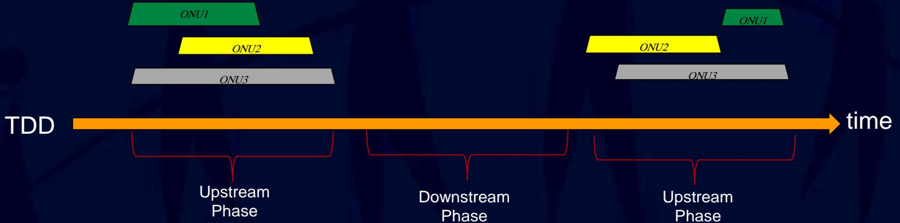
One way to avoid frame fragmentation in upstream for TDD is for CNU to report on frame boundary within each TDD upstream phase
