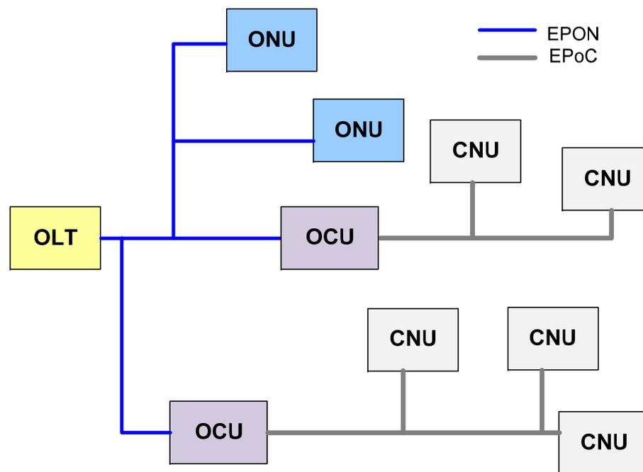
**(b) Integrated EPON / EPoC Plant**
