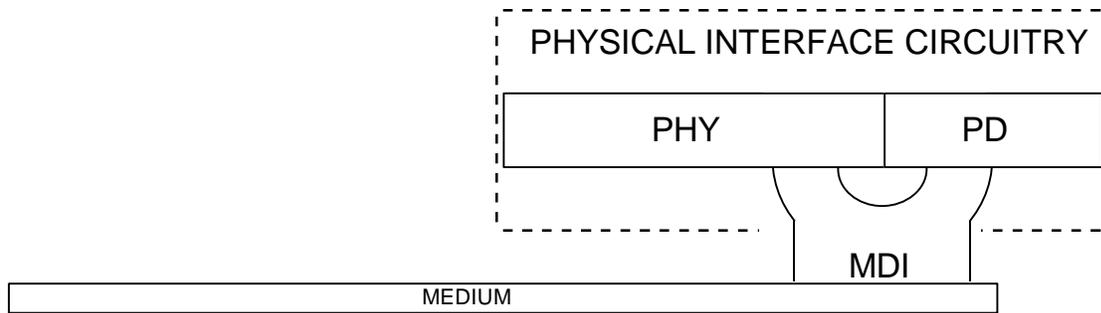
**Figure 33--1--DTE Power via MDI Powered Device (PD) relationship to the Physical Interface Circuitry and the IEEE 802.3 CSMA/CD LAN model**
