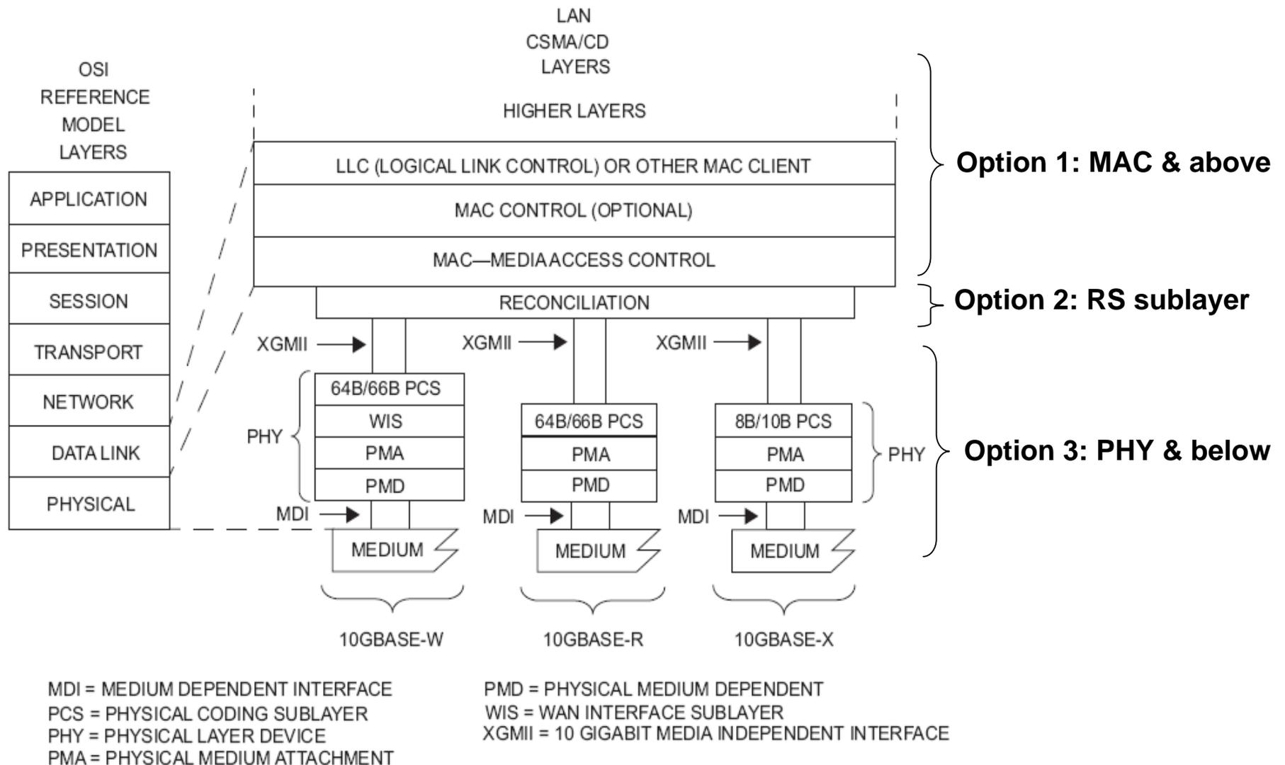
Figure 44–1—Architectural positioning of 10 Gigabit Ethernet
