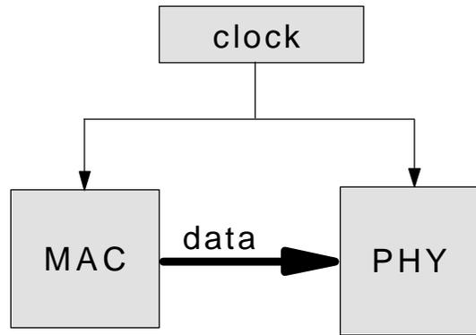
Figure. 1 Option C Clocking Scheme
