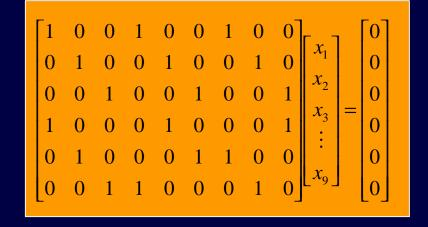
• LDPC codes are binary, linear error-correcting codes, defined by sparse parity check matrices.
