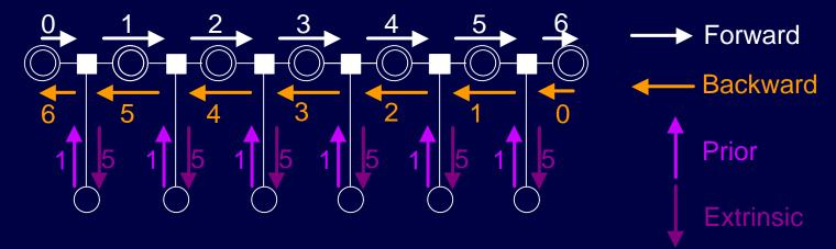
Message-passing gives the correct answer for graphs without cycles. In general, messagepassing does not work for graphs with cycles...
