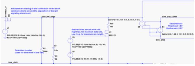
Sink dominant "0" transmission is achieved via M1 and R10. While data discrimination in *Sink\_Data\_RAW* is achieved via a comparator with a threshold of 1.5V and a hysteresis of  $\pm 0.1V$  (E4 & E5). Termination of the data line is done similarly to the source via C3 & R3.
