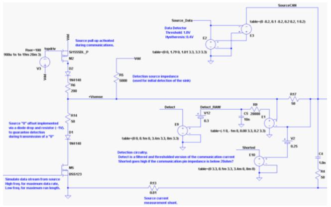
A source pull-up (R6) is activated via M2 and D2 to allow for the desired communications speed. Note that this pull-up (together with D2, D1, R14, and R17) limits communications current to a maximum of 10mA. The transmission of a dominant "0" is achieved via M5, with D1 and R14 limiting the excursion to keep at least 1V of bias in the communications line (for detection purposes). D2 serves to protect M2 in case of a short to the power line.
