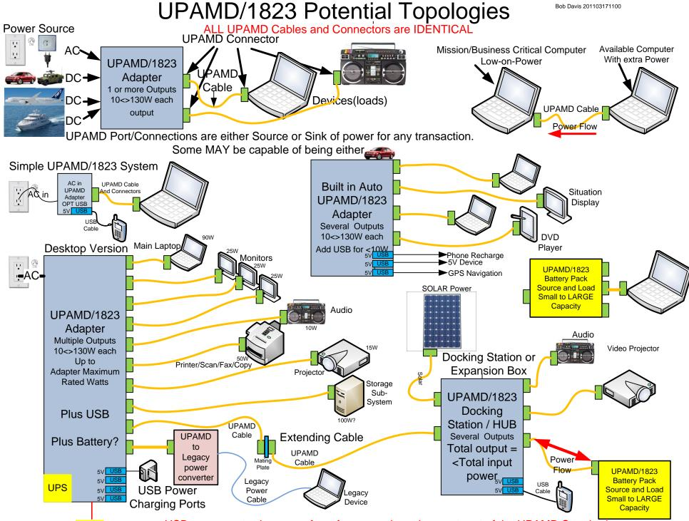
USB power ports shown are for reference only and are not part of the UPAMD Standard Uninterruptable Power Systems (UPS) shown are for reference only and are not part of the UPAMD Standard
