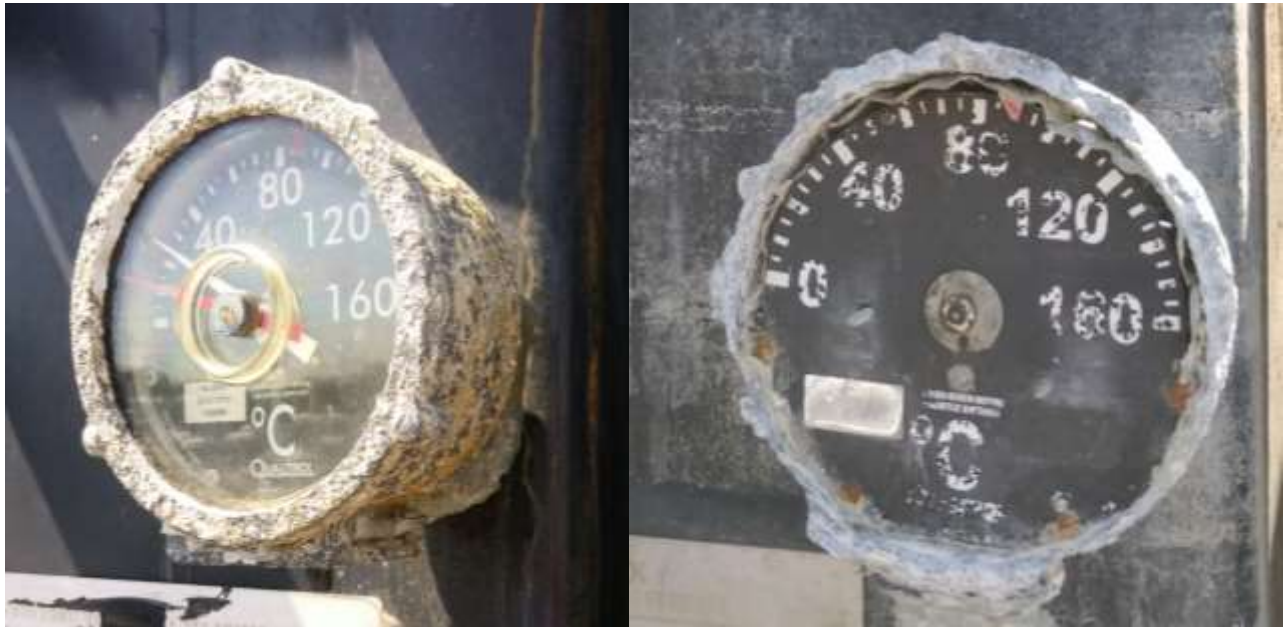
Figure 10: Thermometers with Aluminum Case on Silicon-Bronze Threads
