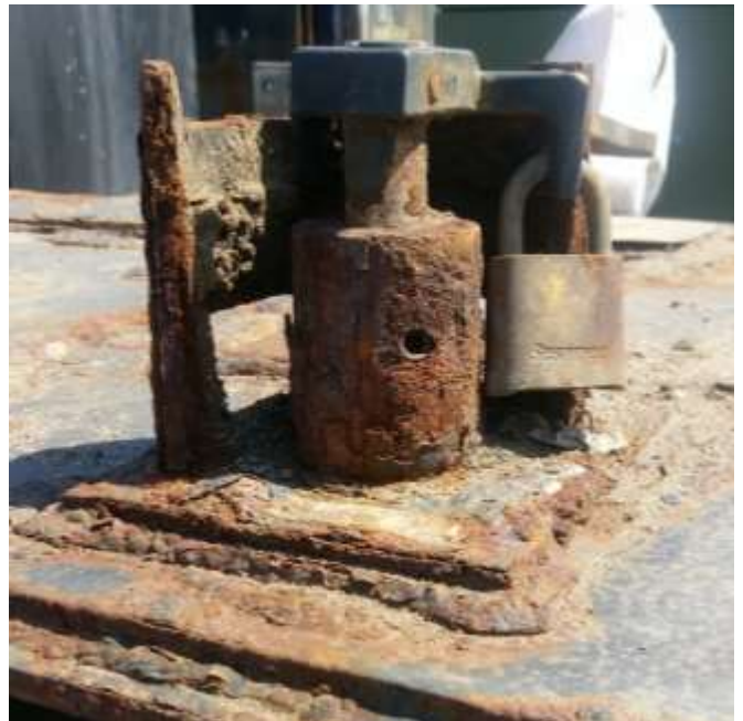
Figure 9: Silicon-Bronze Padlock on Steel
